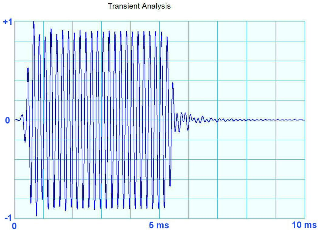
Figure 2 – A 500 Hz pulse 50 milliseconds long as it exits from that I.F.
