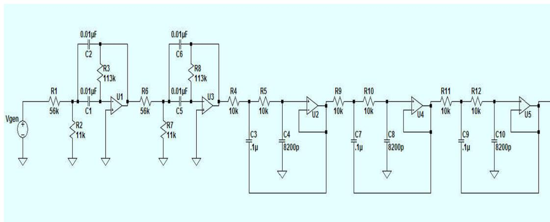
Figure 17 – Schematic of an active equivalent of the filter
