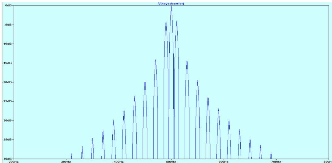
Figure 13 – Spectrum of the pulse when shaped by the five millisecond rise and fall time constraint.
