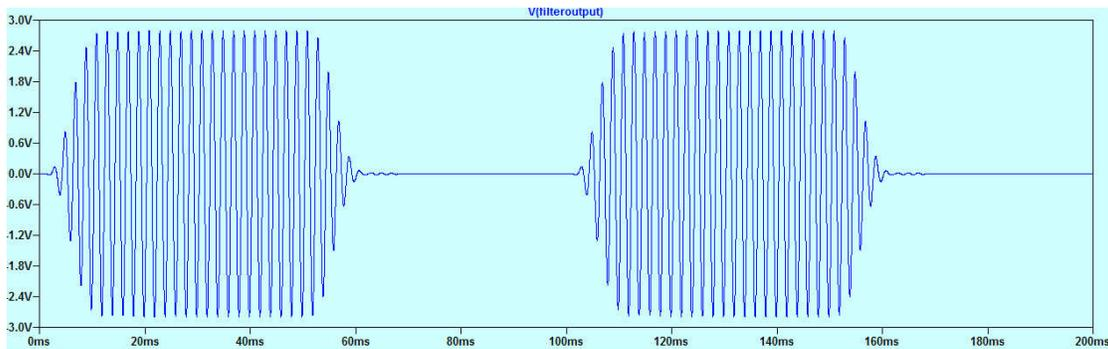
Figure 14 – The narrowband pulse after it has passed through the add-on bandpass filter
