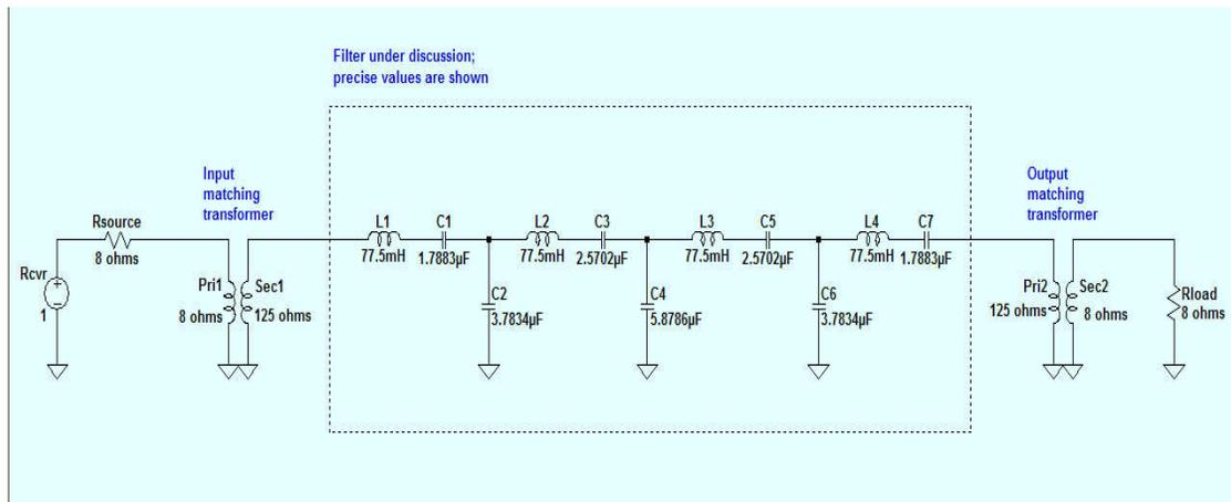
Figure 18 – Schematic of the passive add-on bandpass filter
