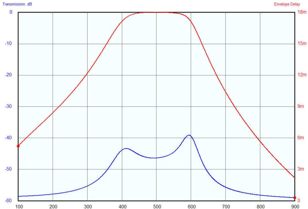
Figure 5 - Magnitude response of the add-on filter (upper plot) and group delay (lower plot)
