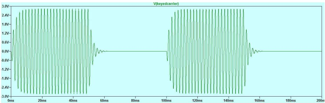
Figure 12 – The narrow banded pulse. The pulse was subjected to a five millisecond rise and fall time
