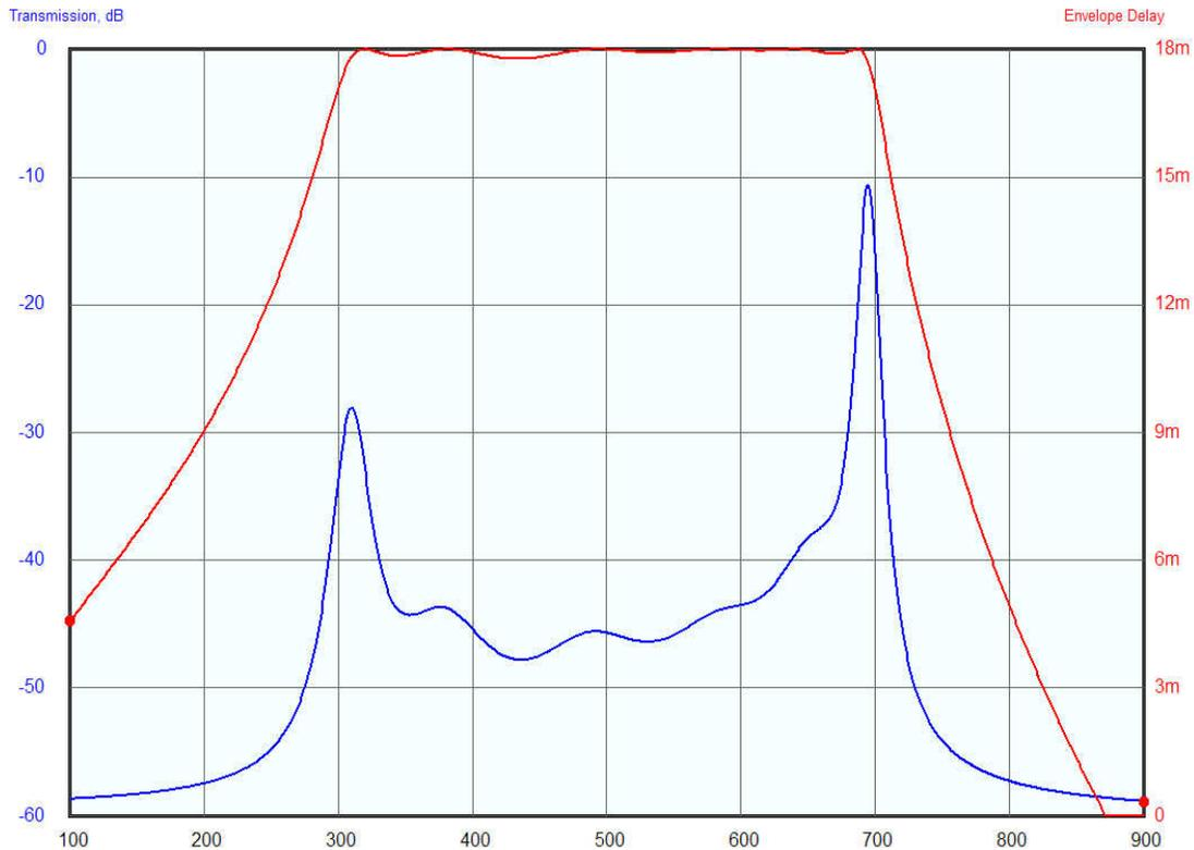
Figure 4 – Magnitude response of the receiver's I.F. strip (upper plot) and the associated group delay (lower plot)
