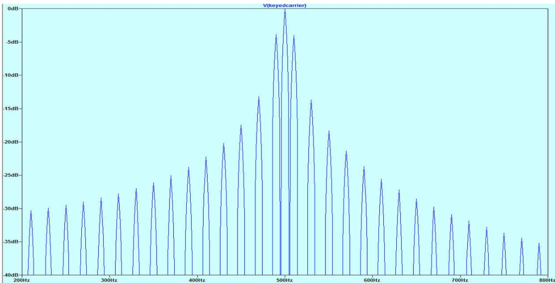
Figure 11 – The spectrum of that raw (unshaped) keyed CW signal
