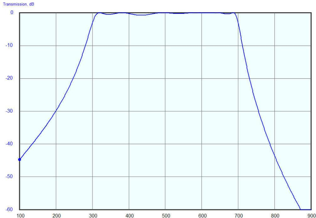
Figure 1 – Response of typical I.F. strip
