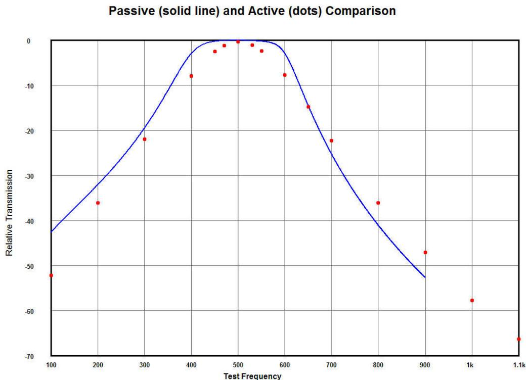
Figure 15 – Responses of the passive version of the filter (solid line) and an active filter approximation (dotted) using a linear frequency scale
