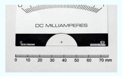
Print a scale and confirm that the mounting hole separation is correct, as shown here by laying the plate on top of the printout.
