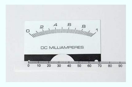
Now measure the separation between the mounting holes (67 mm here). **This must** be an accurate measurement.
