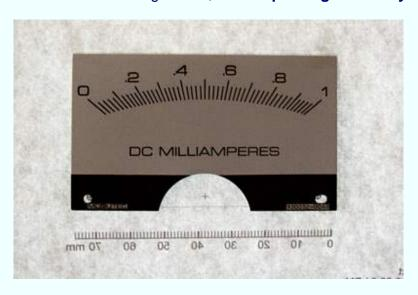
Place the *reverse* side of the metal plate against the non-printed side of the newly-printed scale. (By doing this, the original lettering will not show through the new paper scale.)
